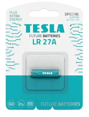
**DESCRIPTION:** Mercury Free Alkaline Manganese Battery, LR27A / Non-Rechargeable **CHEMICAL SYSTEM:** Alkaline Manganese SHELF LIFE: 7 years **NOMINAL VOLTAGE:** 12 Volts **NOMINAL DIMENSIONS:** Ø 7.8 mm × 27.9 mm TERMINALS: Protruded positive(+) and flat negative (-) contacts JACKET: Foil jacket **APPLICATIONS:** All electronic devices, e.g.outdoor bells, car keys, photo equipment. **STORAGE TEMPERATURE:** +10 °C to + 25 °C Should be stored in dry and cool place. **NOMINAL WEIGHT:** 5,1 g
