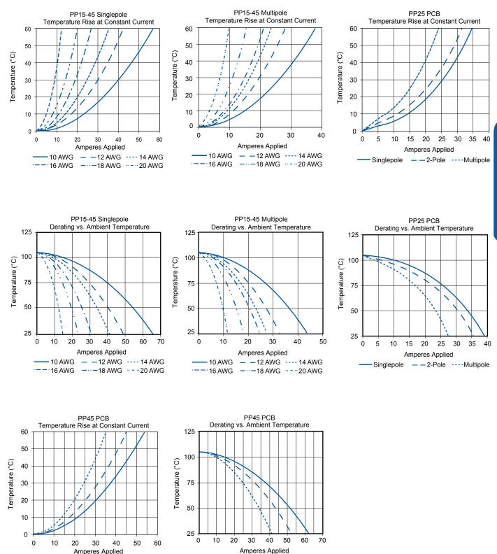
NOTE: Temperature rise charts are based on a 25°C ambient temperature. PP25 PCB charts based on 0.002 in² foil on board side, mated to #12 AWG conductor on wire side. PP45 PCB charts based on #10 AWG equivalent copper foil on board side, mated to #10 AWG conductor on wire side.
