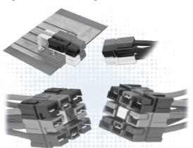
PP15-45 series are the smallest Powerpole® housings. They can be used for wire-to-wire or wire-to-board applications. Wire sizes from #20 AWG (0.75 mm²) to #10 (6 mm²) offer power capabilities up to 55 amps per pole. Finger proof housings and the ability to incorporate first-mate last-break ground connectors enhance the capabilities of this Powerpole® series.
